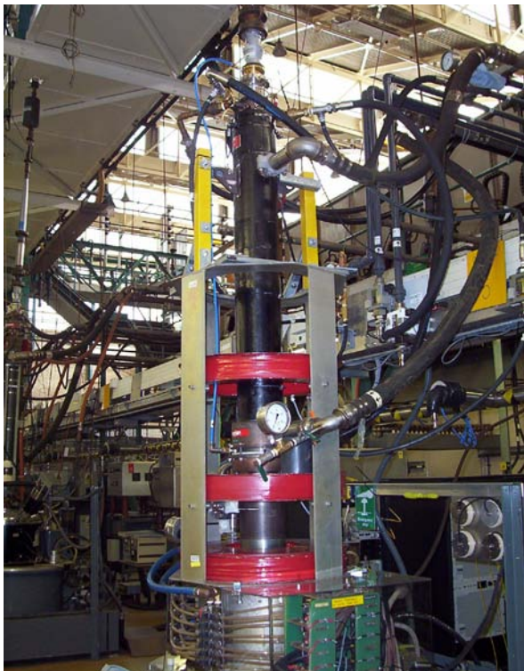
▲ The 28 GHz gyrotron on the MAST spherical torus device for use in the plasma start-up experiments.
