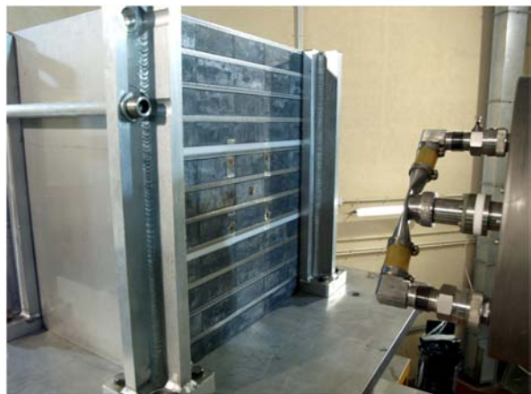
▲ Direct measurement of tritium production in irradiated lead-lithium walls.
