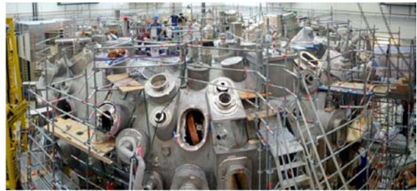
▲ The Wendelstein 7-X will be the first stellarator to combine improved confinement with plasma equilibrium and stability. The first plasmas are expected by 2015.
