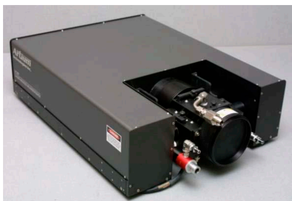
▲ This innovative optical instrument measures concentrations of black carbon in diesel engines.
