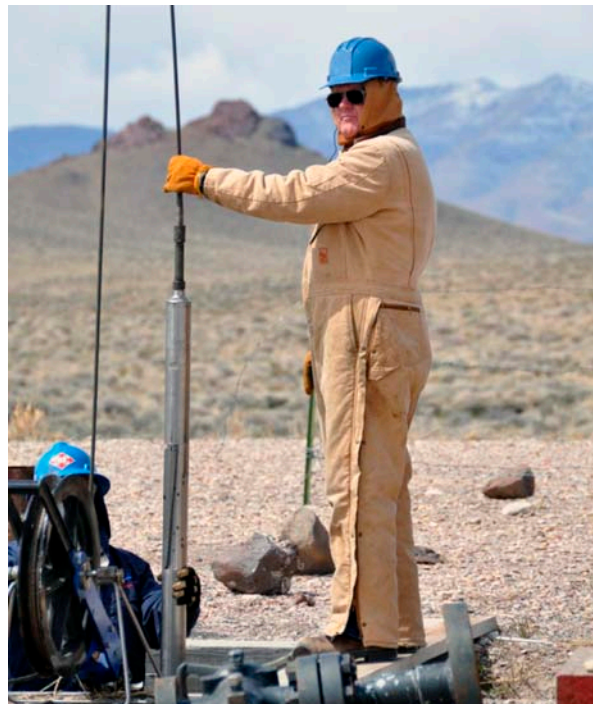
▲ Participants in the GIA study logging (testing) a geothermal well to determine how to reduce costs.
