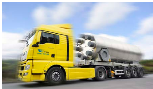
▲ Heat recuperated from a waste incinerator is transferred to an industrial drying processor using a thermo-chemical storage tank.
